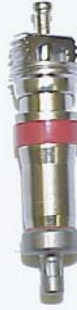
70-HT: LARGE BORE VALVE CORE: Opening Pressure: 35 psig Cup Seal Material: Silicone
