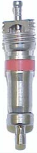
70-HV LARGE BORE VALVE CORE: Opening Pressure: 35 psig Cup Seal Material: Viton
