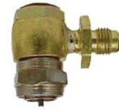
9044 Lock Chuck (Standard Bore) .307-32 thread and .375-24 side hose connector. Maximum operating pressure of 3000 PSI
