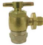
9043 Lock Chuck (Standard Bore) T-Handle with .307-32 thread and .375-24 side hose connector. Maximum operating pressure of 3000 PSI
